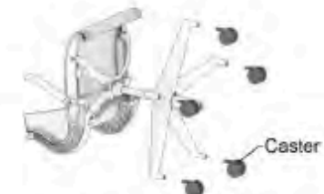
2.1. Grasp and pull to remove Casters from the Base.
